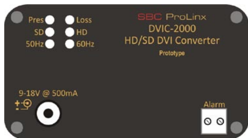
Front panel with power connector
