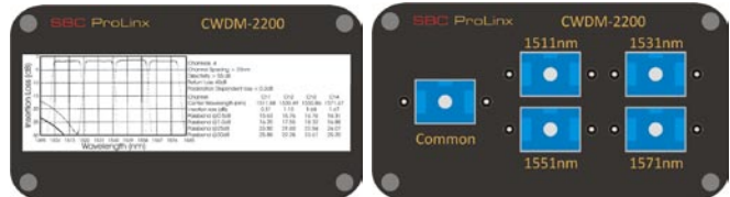
CWDM 2200 Front and Rear panels
